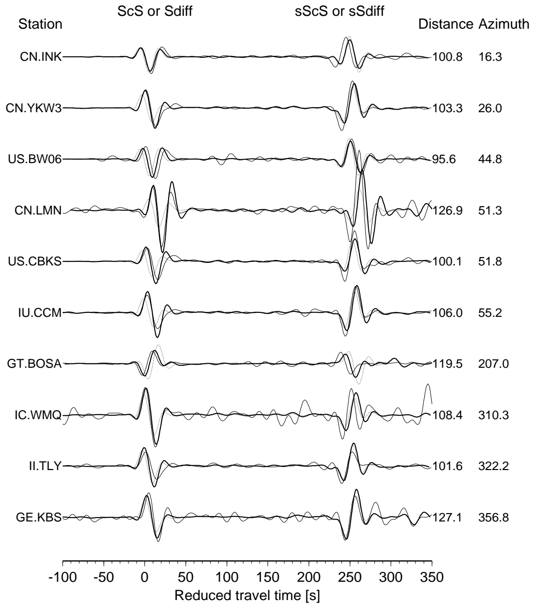
Figure 2.11: Comparison between data (thin line), synthetics in PREM (dotted line) and synthetics in SAW24B16 + PREM (bold line).
