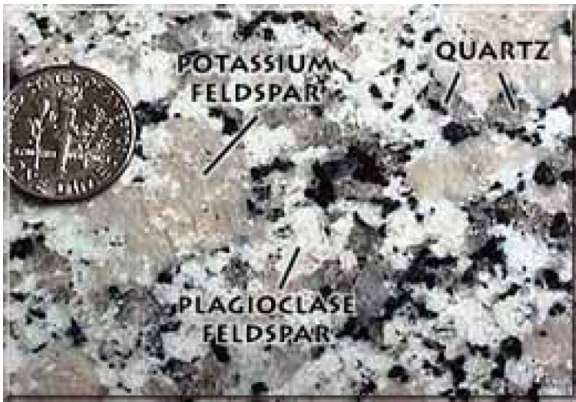
Figure 2.22. A close-up photo of granite. Notice that it is made up of interlocking large crystals. The large crystals form when molten rock is allowed to cool slowly deep within the earth. When molten rock is erupted onto the surface by volcanoes, it cools quickly, so volcanic rocks mostly lack large crystals. The labels show the names of some of the minerals in granite.
