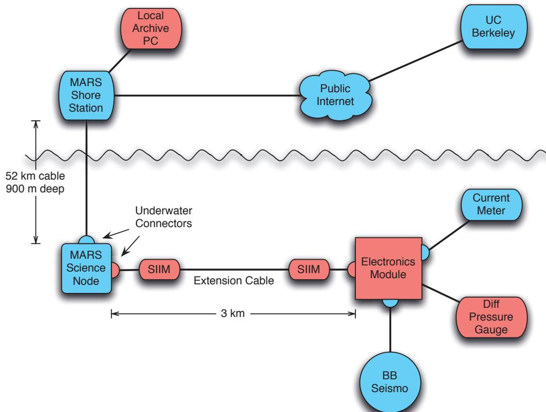
▲ **Figure 2.** Components of the cabled observatory: the MOBB system integrated into the MARS network. MARS-provided components and components of the current MOBB installation are shown in blue. Components shown in red are those installed or replaced as part of our current NSF-funded upgrade. When the data arrive at UC Berkeley, they will be incorporated in the joint UCB/USGS real-time earthquake notification system and made publicly accessible online at the NCEDC.
