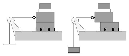
Figure 10. DST box at start of test (left) and weight is added to cause displacement (right).
