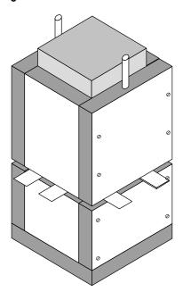
Figure 9. Assembled DST box with shims in place.
