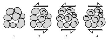
Figure 1. The packing of particles can change radically during cyclic shear; (1) a large hole is maintained by the particle interlocking; (2) a small counterclockwise strain causes the hole to collapse; (3) large shear strain causes more holes to form; (4) holes will collapse when the strain direction is reversed (*Youd*, 1977).
