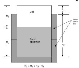
Figure 11. Determining the height of the sand specimen.
