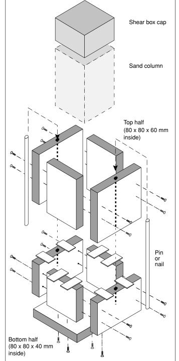
Figure 8. Exploded view of Direct Shear Test box; light gray volume indicates sand.
