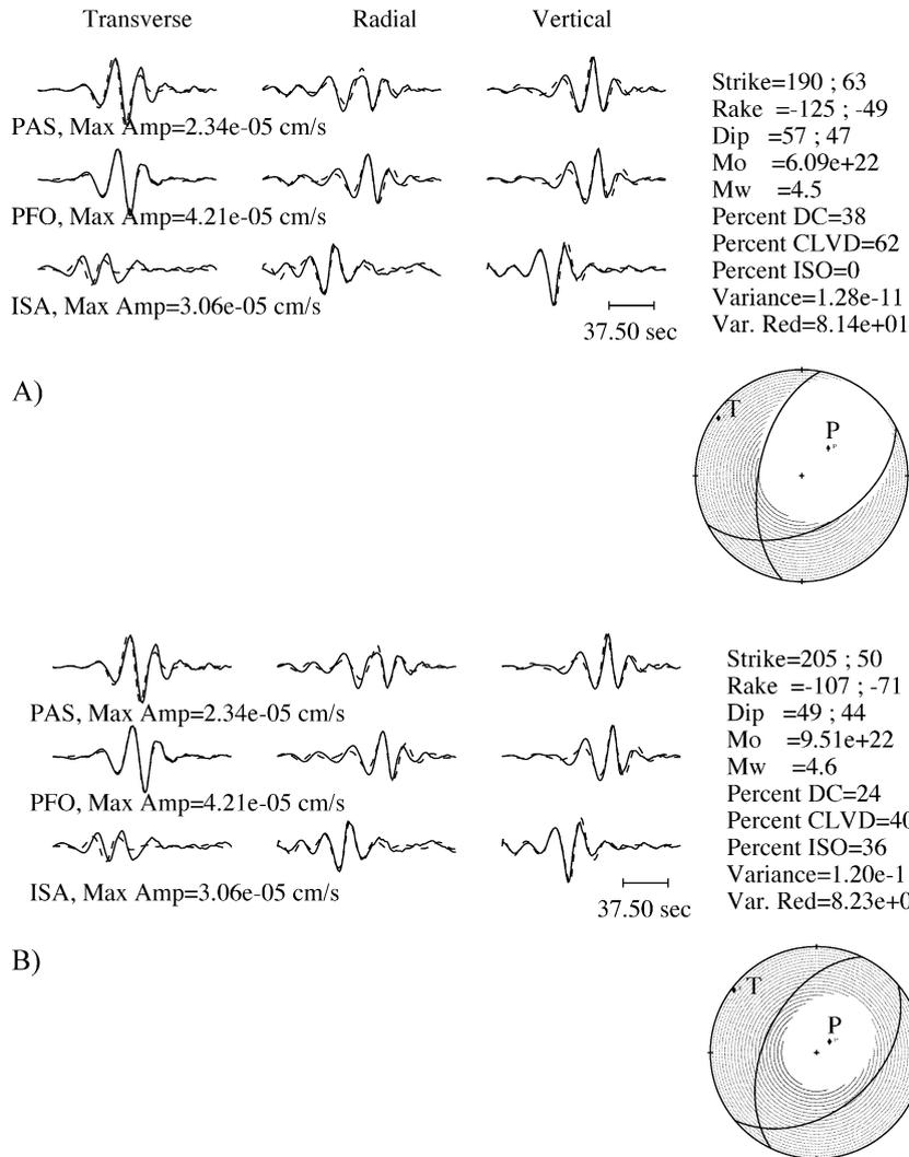
Fig. 5. Same as Fig. 4 for the MONTELLO explosion.
