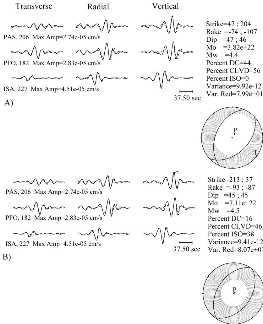
Fig. 6. Same as Fig. 4 for the BEXAR explosion.
