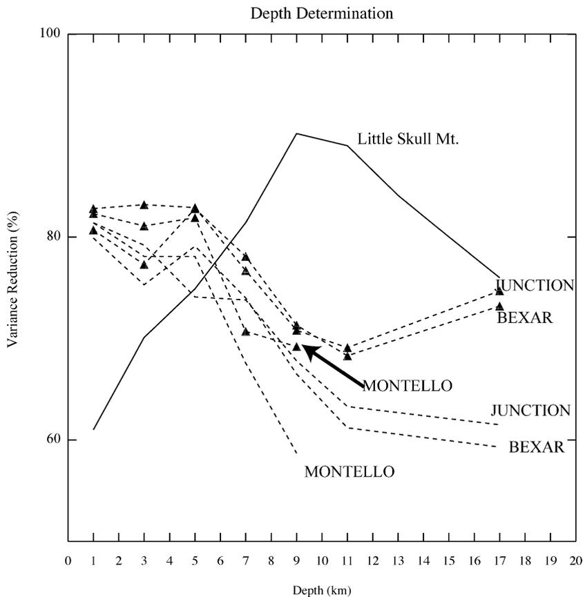
Fig. 3. The variance reduction vs. source depth for the deviatoric inversions are compared for the Little Skull Mountain Earthquake (solid line), and the JUNCTION, MONTELLO and BEXAR nuclear explosions (dashed curves). The dashed curves with symbols show the variance reduction vs. source depth for the full-moment tensor inversions for the three nuclear explosions.
