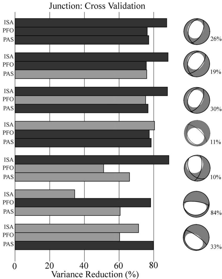
Fig. 8. Cross-validation results. The variance reduction for each three-component station is plotted for single-, two- and three-station DEVMT inversions. The black bars show the variance reduction for the stations used in the inversion, and the gray bars show the variance reduction for stations whose waveforms were predicted by the derived solution. On the right, the P-wave radiation pattern is plotted together with the percent double couple.
