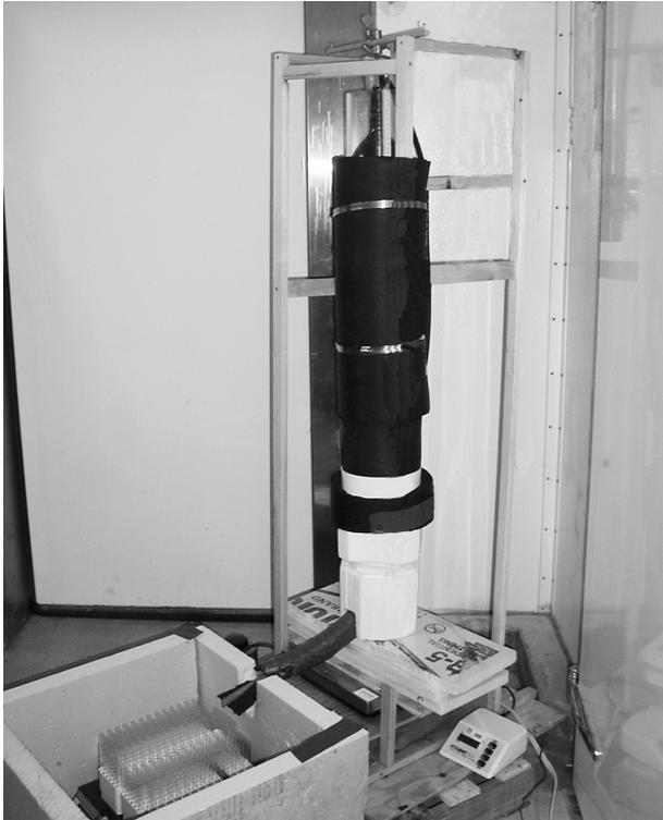
**Figure 1.** Laboratory snow column experimental setup.
