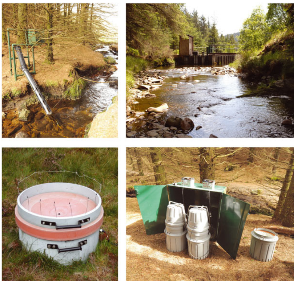
Figure 1. Photographs of sampling sites and instrumentation. Clockwise from upper left: (a) sampling point on the Upper Hafren with protective housing for sampling tube; (b) sampling point on the Lower Hafren, just upstream from the flow gauging structure; (c) duplicate Xian automatic samplers and protective enclosure at the Upper Hafren sampling site; and (d) continuously open 7-hourly rainfall collector (57.5 cm diameter) in short grass vegetation near the Upper Hafren catchment
