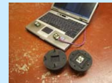
Fig. 10. Wireless sensor ball measures acceleration and orientation.
