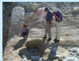
Fig. 4. The erodible slabs are secured by a heavy steel frame, upstream of a check dam. After a debris flow event, they are uncovered and photographed.
