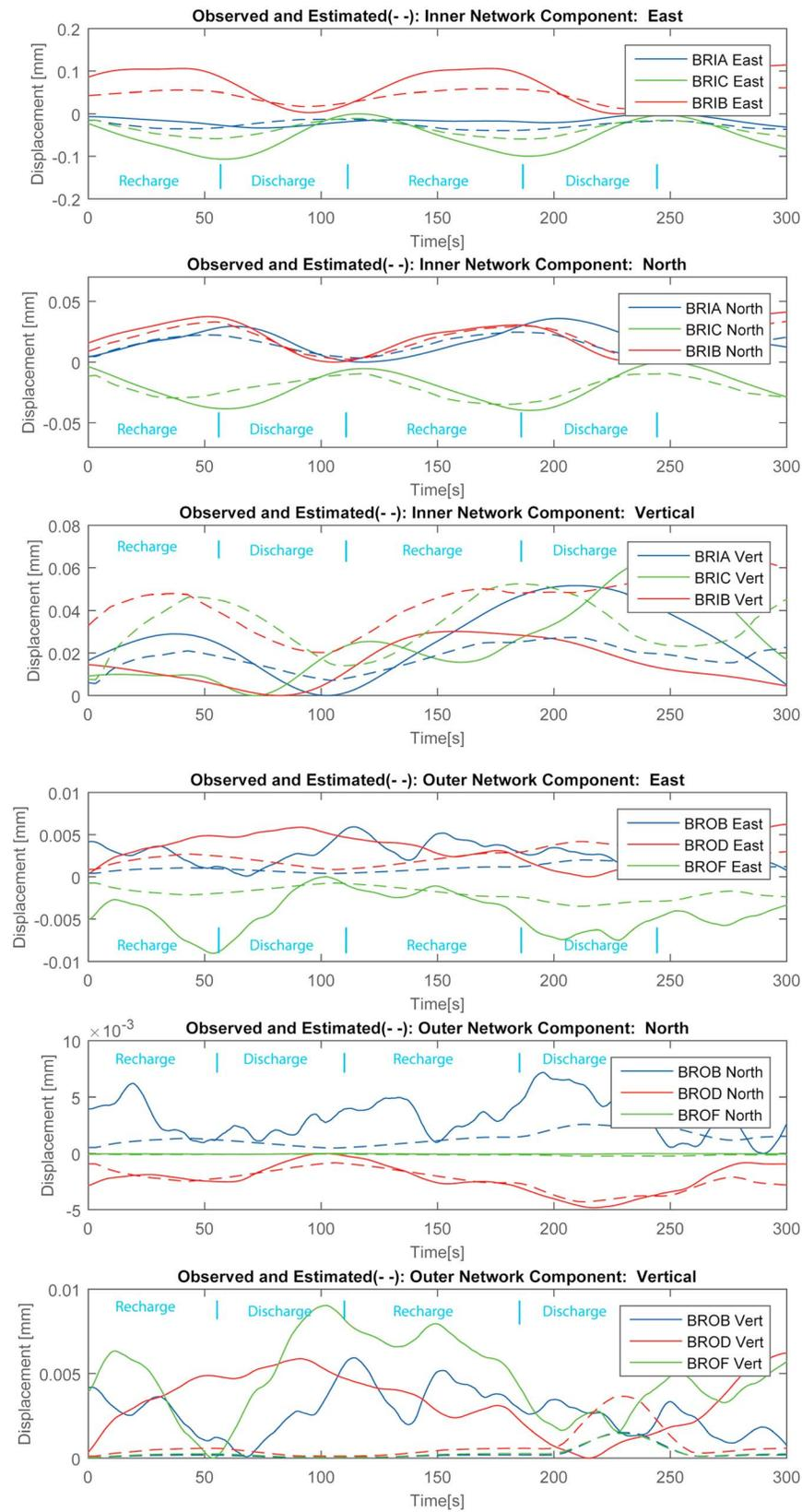
**Figure 6.** Synthetics and observed time series of displacement for the internal network stations: (a) east, (b) north, and (c) vertical, and for the outer network stations: (d) east, (e) north, and (f) vertical.
