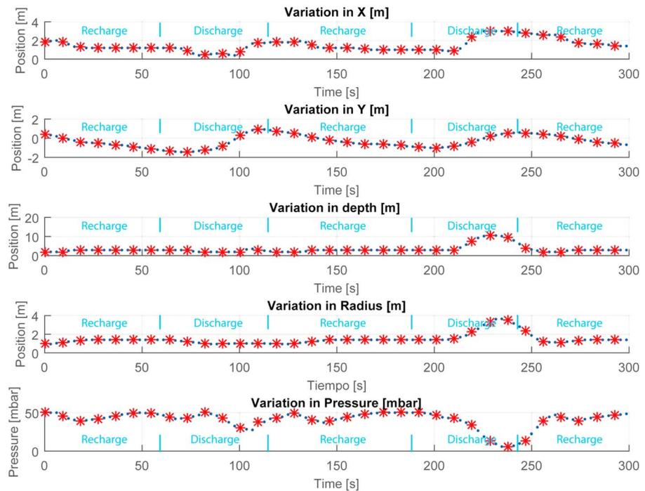
**Figure 5.** Variation of the optimal parameters covering 300 s. The cyclicity in all parameters is apparent. The best models fit well the large-amplitude horizontal displacements at the inner stations but not the vertical displacements nor the displacements at the distant stations. The blue dots are parameters estimated every 2 s, and the red asterisks are the ones estimated every 6 s. The models shown in Figure 4 are plotted directly from these parameters.
