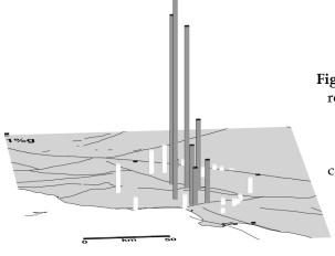
Figure: Perspective map of the Los Angeles area showing recorded peak acceleration (vertical bars) between 9 and 10 sec after the Northridge earthquake. Grey bars are predominantly horizontal motion, white are the predominantly vertical P-arrivals which arrive first but cause little damage. The sites above the fault plane start to experience their peak ground motion in this time window, 3 sec after a magnitude estimate can be made from the P-arrivals at the same stations.
