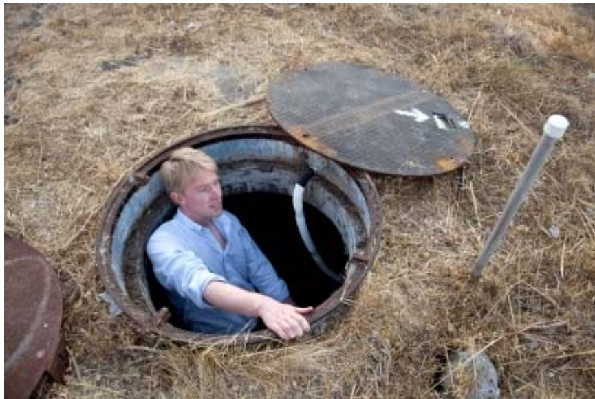
Most of the 285 sensors that make up the California Integrated Seismic Network are buried underground, like this one in an old water tank in Ohlone Park, in Hercules.
