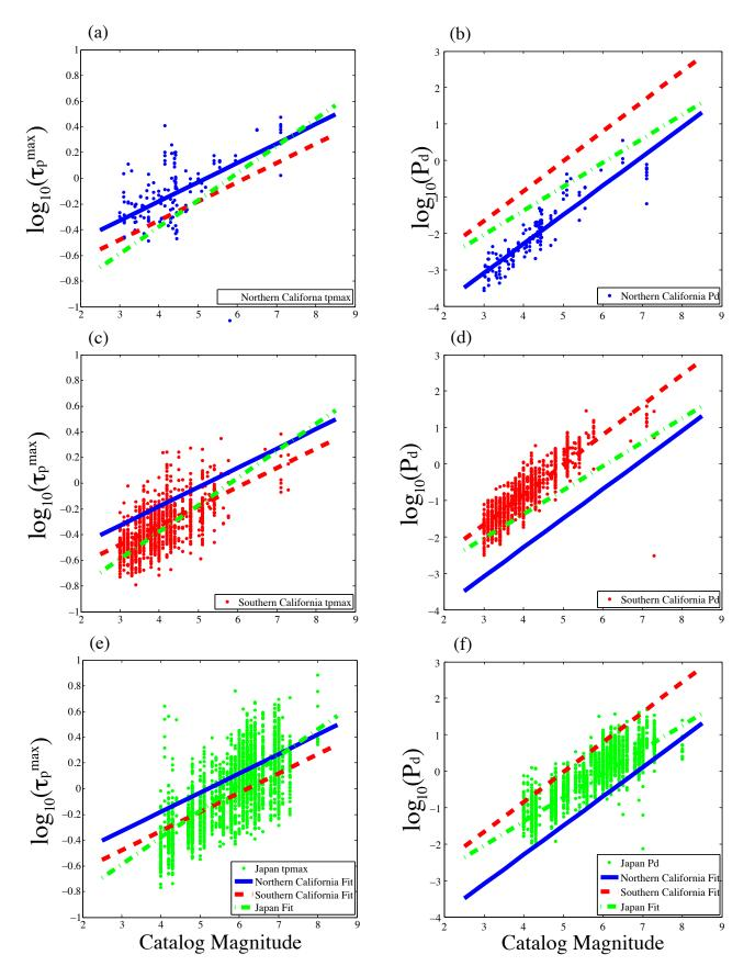
Figure 3.2. Scaling relations. (a) τpmax, northern California; (b) Pd, northern California; (c) τpmax, southern California; (d) Pd, southern California; (e) τpmax, Japan; (f) Pd, Japan. Circles are individual station observations of τpmax or Pd. Lines are regional scaling relations defined by the linear best fit to the data. The best-fit linear relations for all three regions are shown on all plots.
