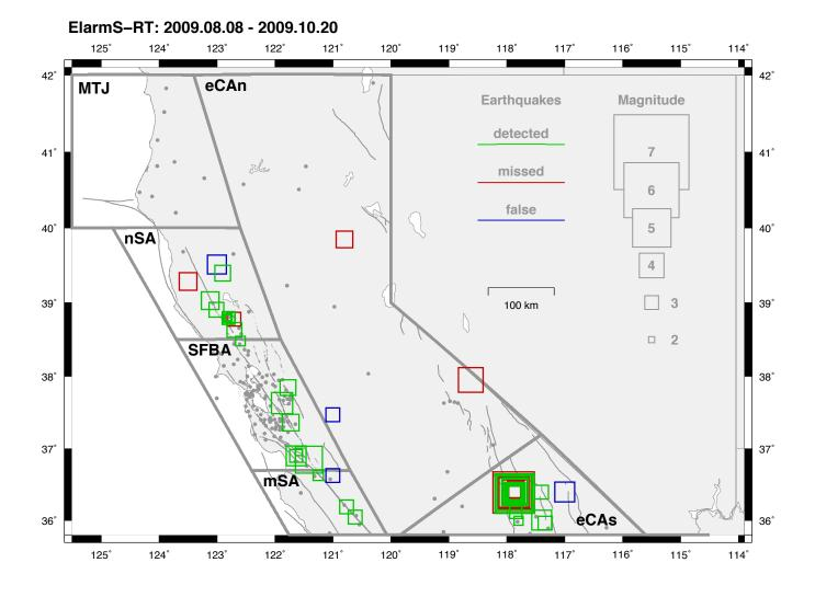
Figure 3.4. Map showing all ElarmS-detected earthquakes with M>3, and all false and missed alerts in Northern California, during a ten-week test period from 8 August 2009 until 20 October 2009. Green, red, and blue boxes are detected, missed, and false alerts, respectively. Grey dots are seismic stations.
