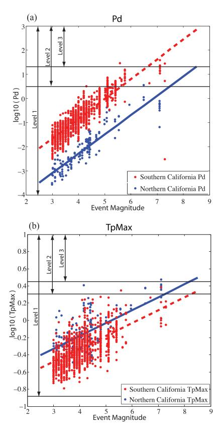
Figure 4.3: Threshold values for (a) Pd and (b) TpMax P-wave parameters. Values must be within level 1 for a trigger to be associated with an existing event or used to generate a new, 3+ station event. Values must be within level 2 to generate a 2 station event, and within level 1 to generate a single station event. More information about the Pd and TpMax magnitude scaling relations can be found in Brown, et al., 2009.
