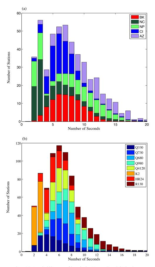
Figure 3.3. A stacked histogram of latencies by (a) network, and (b) data logger type. Both histograms are truncated at 20 seconds for clarity, but the long tail to the histogram continues, with columns of 0-2 data points, up to as much as 200 seconds.
