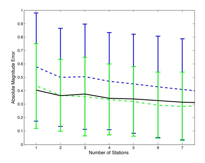
Figure 2.4: Effect of number of stations on the accuracy of magnitude estimates. The blue dashed line is the average error in magnitude estimates made using only maximum predominant period,  $\tau$ pmax. The green dashed line is the average magnitude error using only peak displacement, Pd. The solid black line is the error when the two estimates are averaged.
