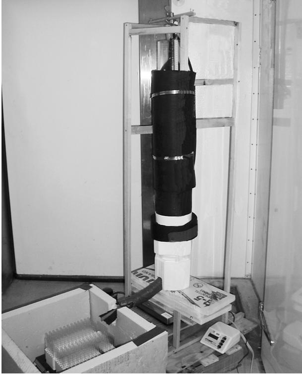
**Figure 1.** Laboratory snow column experimental setup.
