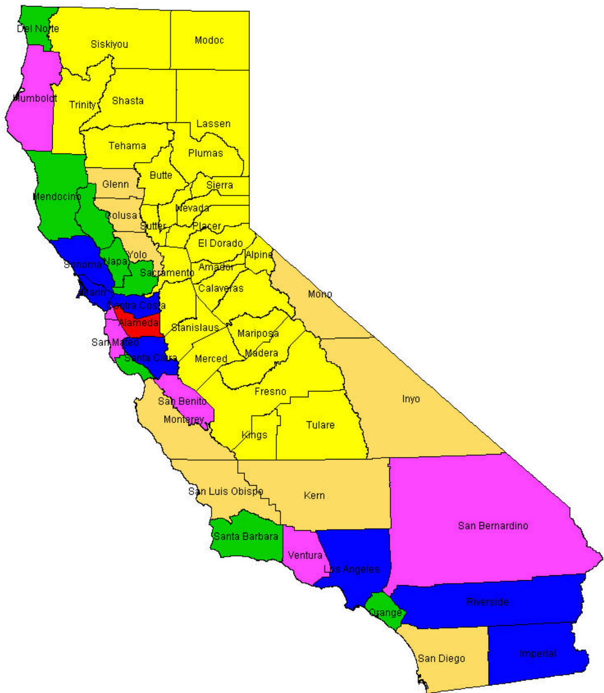
Figure 22 - Annual building damage economic loss as percentage of building replacement value by county, based on the 2002 PSHA maps, weighted average soil, with liquefaction effect.
