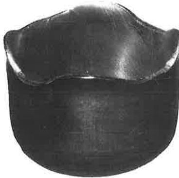
Fig. 3. Cup formed by deep-drawing a rolled sheet of aluminum. The 'ears' are evidence of texture-caused anisotropy. [Courtesy Marc Verdier]
